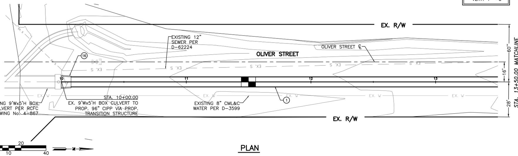
\*FOR CIPP—WHERE PIPE VELOCITIES ARE GREATER THAN 10 FPS BUT NOT MORE THAN 20 FPS, A 140 DEGREE SEGMENT OF INVERT SHALL BE THICKENED 2 INCHES IN WALL THICKNESS AS A "SACRIFICIAL CONCRETE"
