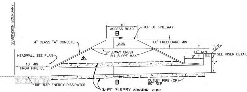
**SECTION A-A: SECTION THROUGH EMBANKMENT**
