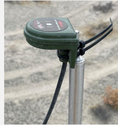
Photo 6. Bat detector microphone extended vertically.
